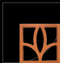
49 (204mm x 204mm) Lily Jaali Size : 8"x8" Per 100 Sq. Ft. 225 Nos 1 Sqm. = 25 Nos Weight Kg/Pc : 2.5
