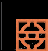
46 (204mm x 204mm) Pearl Jaali Size : 8"x8" Per 100 Sq. Ft. 225 Nos 1 Sqm. = 25 Nos Weight Kg/Pc : 2.5
