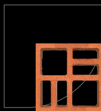
45 (204mm x 204mm) Square Jaali Size : 8"x8" Per 100 Sq. Ft. 225 Nos 1 Sqm. = 25 Nos Weight Kg/Pc : 2.5
